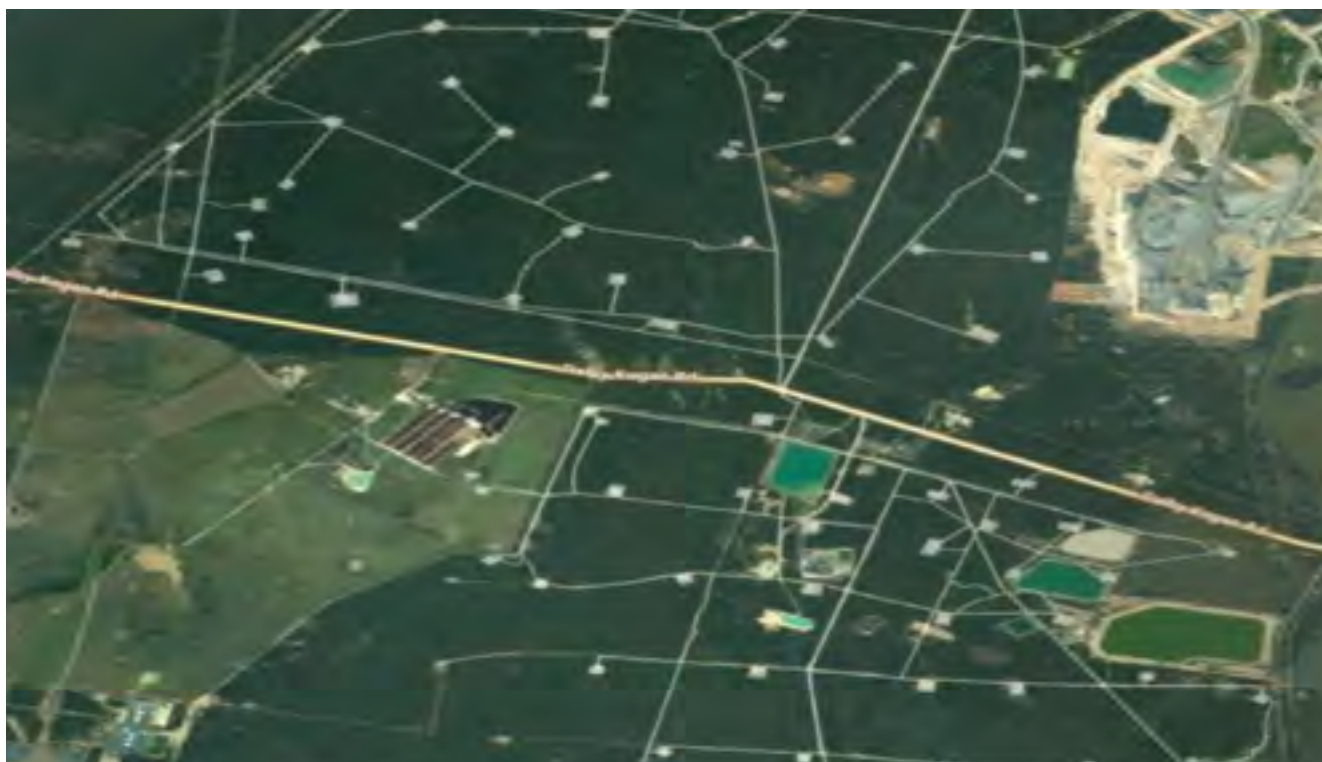
Figure 3-1 Demonstration of the broader impacts of multiple CSG wells in the landscape with the roads and other infrastructure in a CSG field near Dalby State Forest, southern Queensland. Scale widthways: 6.8 kilometres. Source: Eco Logical Australia 2013
