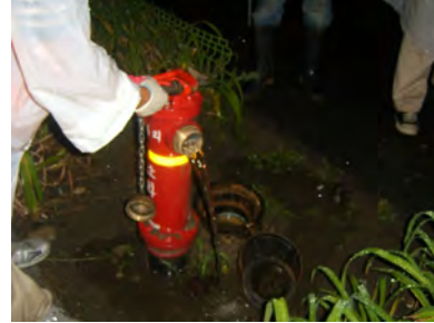
[Performing the Test: Checking Water Quality at Hydrant or Water Tap]
