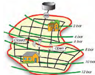
[Opening the Boundary Valve between Two Pressure Zones]
