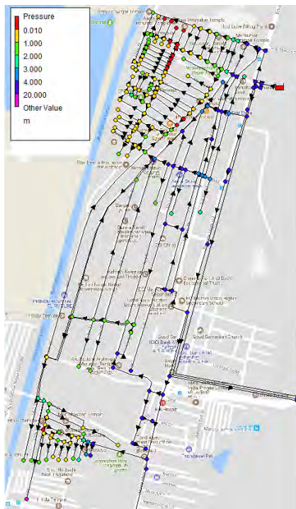
[Hydraulic Modeling Based on Measured Data]
