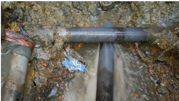
[Pipe Burst caused by Two Pipes Contact]
