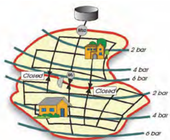
[Pressure Profile after Re-establishment of Zones]
