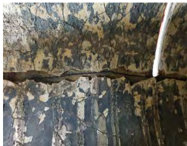
[Pipe Burst Cased by Poor Material in DCIP]
