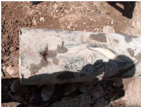
[Outside and Inside of Pipe Broken by External Force]
