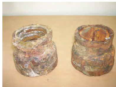
[Corrosion of Pipe Accessories]
