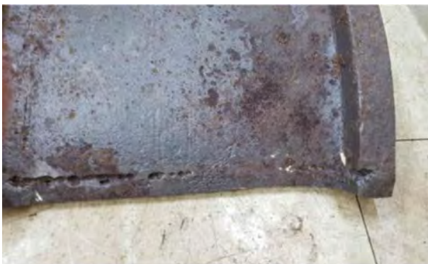
[Unreliable Casting Materials in DCIP]
