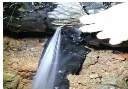
[Leakage Caused by Corrosion in Metallic Pipe]
