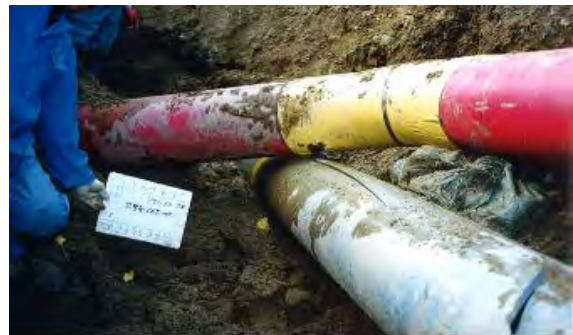
[Pipe Burst caused by Two Pipes Contact]
