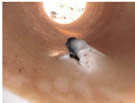
[Outside and Inside of Pipe Broken by External Force]
