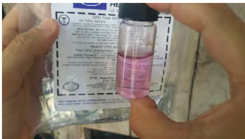
(c) Water Quality Measurement (Residual Chlorine)
