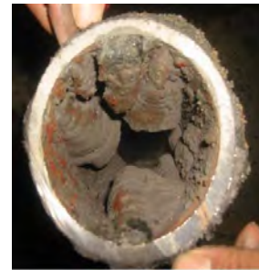
[Internal Damaged Coating and Lining, Tubercle, and Scale in Metallic Pipe]
