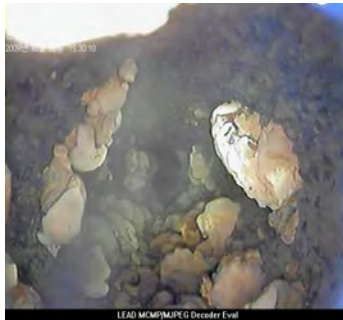
[Internal Damaged Coating and Lining, Tubercle, and Scale in Metallic Pipe]
