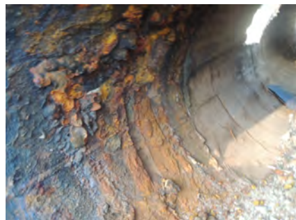
[Internal Corrosion in Metallic Pipe]
