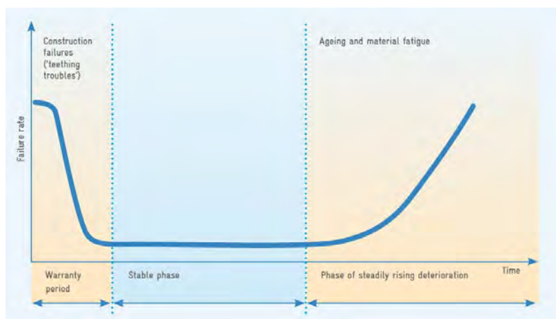
[Typical Behavior of Failure Rate in Pipes]
