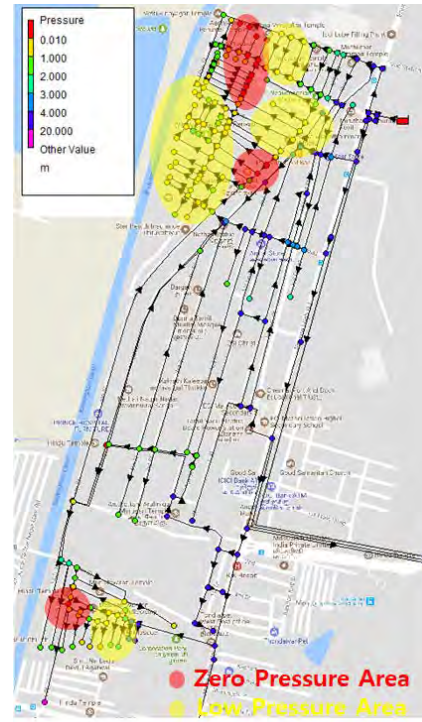
[Hydraulic Modeling Based on Measured Data]
