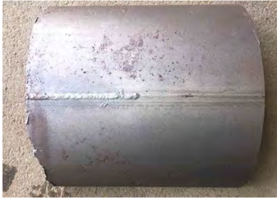
[Poor Welding in SP]
