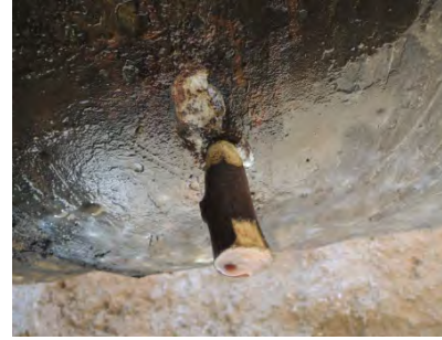
[Improper Repair Using a Wooden Needle]
